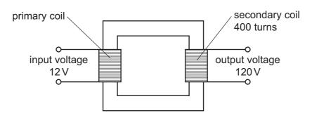
How many turns are on the primary coil of the transformer?
