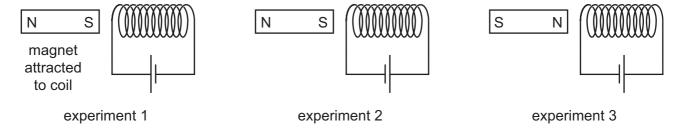
In experiment 1, the magnet is attracted to the coil.
