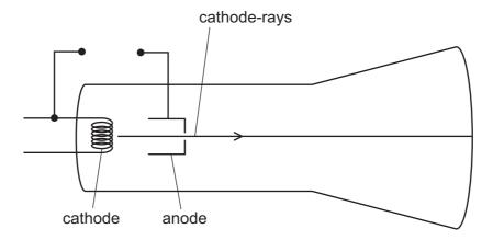
Which electrode should be heated, and which electrode should be positive?
